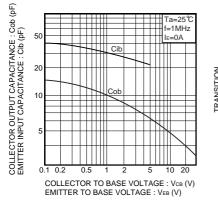
Fig.7 Input-and-output capacity vs.voltage characteristic
