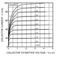
Fig.2 Ground emitter output characteristics
