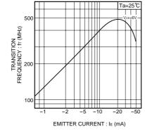
Fig.8 Transition frequency vs.emitter current
