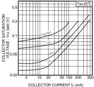
Fig.5 Collector-emitter saturation voltage
